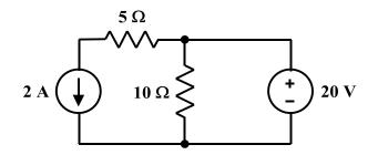
a. How much power does the  $5\Omega$  resistor absorb?
